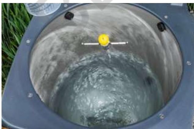
Complete rinsing of induction hopper up to under the cover edge with a total of four WallCleaner nozzles.
