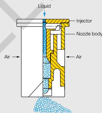
Injector can be removed without tools
