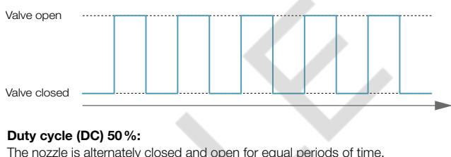
An example: With a duty cycle (DC) of 50%, the applied quantity for nozzle size 06 (gray) corresponds to the quantity of a nozzle size 03 (blue) without PWM. Nozzles are ideally used with a duty cycle (DC) of 30%–100%.
