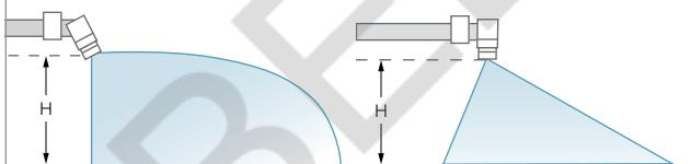
OC nozzle tips fitted in individual or double swivel joints (see Page 128) permit adjustment to any angle. Wide and narrow spray jet widths can be achieved in this way.
