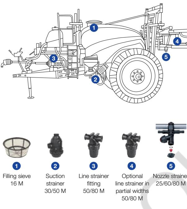
Scheme for selecting the mesh size using the example of a sprayer for viticulture and orchards:
