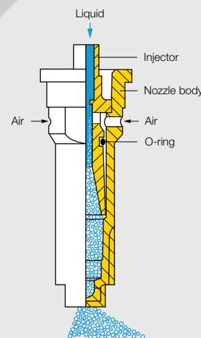
Injector can be removed
