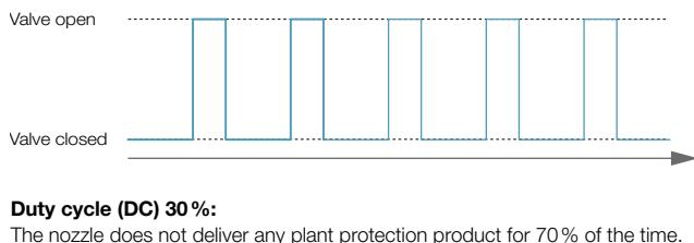
The PWM system can compensate for an excessively large nozzle size by means of a lower duty cycle of 50%–30%, for example, and a reduction in the pressure range. The risk of more uneven distribution of the liquid in longitudinal and lateral direction as well as lower wetting due to the coarser droplet spectrum must be taken into account. The distribution may not be optimal particularly at higher speeds above 10 km/h and with a duty factor of less than 40%.
