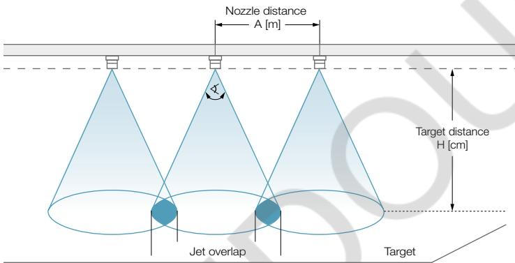
Hollow cone nozzles must be arranged so that the jet cones just overlap shortly before the target surface.
