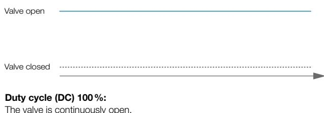
The duty cycle (DC) specifies the time ratio between open and closed valve as a percentage. It is an important variable for good lateral and longitudinal distribution of the sprayed liquid. The valve is open continuously with a duty cycle of 100% – like with conventional nozzles. If the duty cycle is reduced to 50%, the flow rate is also halved – with a constant pressure.
