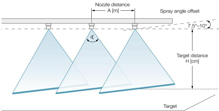
In order to avoid mutual spray jet interference, the jet plane of flat spray nozzles is rotated by about 7.5° to 10° with respect to the pipe axis. This takes place automatically with Lechler diaphragm valves and eyelet connectors with TWISTLOC/MULTIJET bayonet cap. The Lechler nozzle aligner gauge (Order no. **065.231.02.00.00**) is available for systems with screw/union nut fastening.
