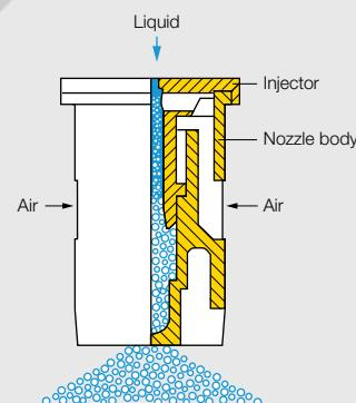
Injector can be removed
