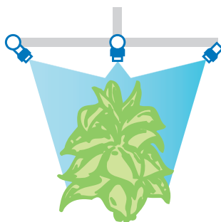
Three Spray Tips Per Row Spacing
